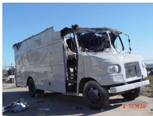
Truck explosion due to improper battery transport
